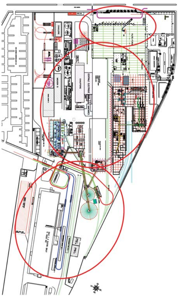
Fig. 15: From right to left: delivery/bulk loading – production – shipping
